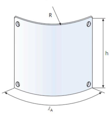
Minimum bending radius (R) = 200 mm
